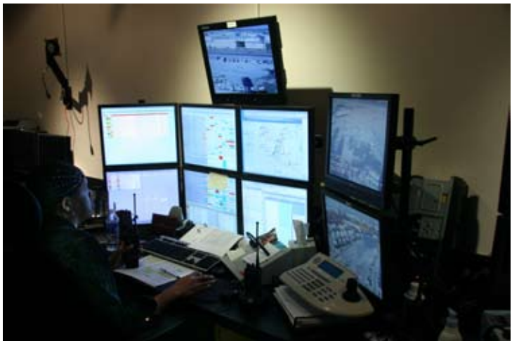
In addition to displays with details for orders in process, trucks en route and the condition of the trucks' individual loads of ready-mixed concrete, the dispatcher can watch truck movements in the batch plants using cameras that send video to several monitors.
