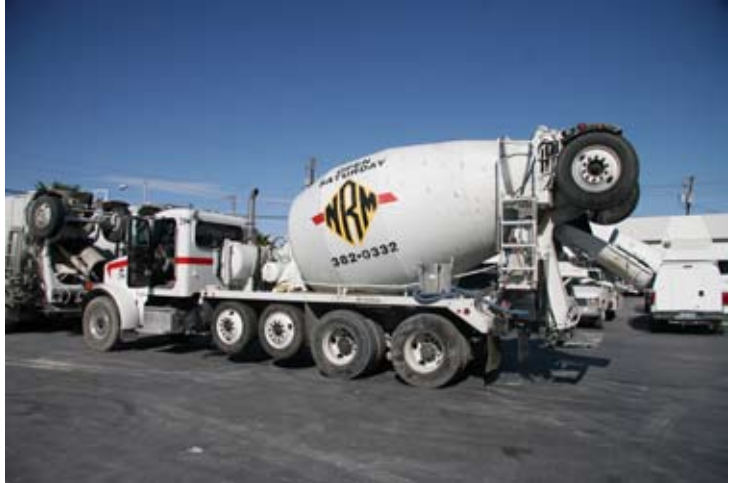
Each Nevada Ready Mix delivery truck is equipped with a two-way mobile radio and a modem that links it with a mobile data system and the company's host computer, plus a computer display for use by the driver.
